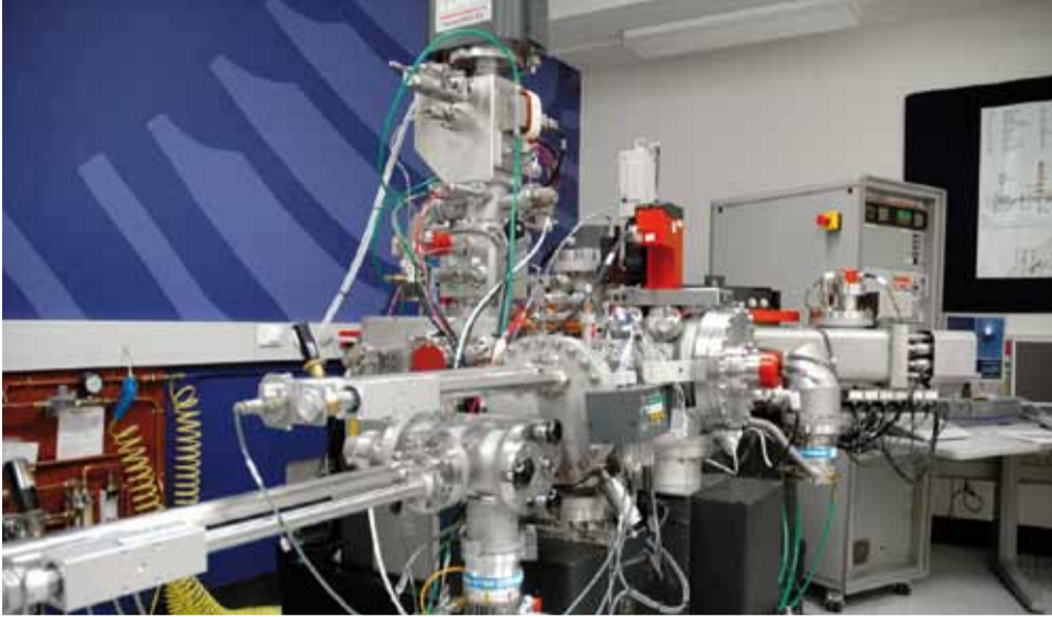
The Cameca NanoSIMS 50 at the Centre for Microscopy, Characterisation and Analysis at the University of Western Australia. This AMMRF flagship instrument is the only one of its kind in the southern hemisphere.
