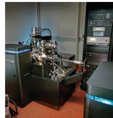
One of the AMMRF's flagship instruments: the Imago wide-field-of-view laser atom probe (LEAP3000) is unique in the Southern hemisphere.
